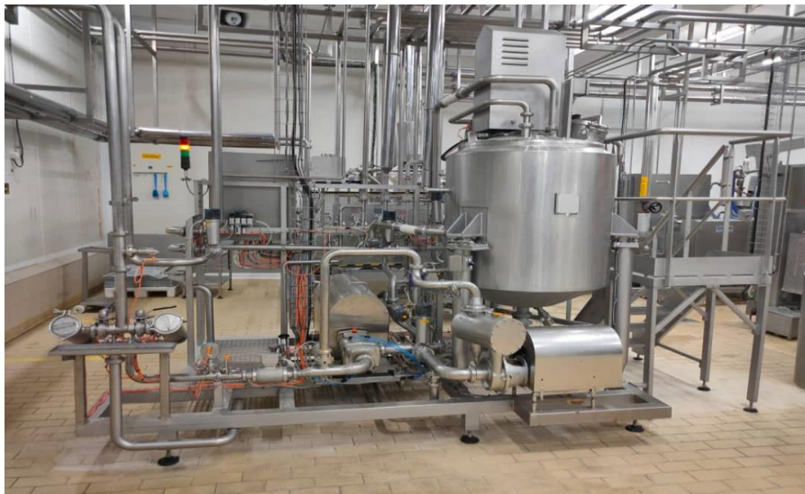
Figure II. 1: Skid de crémage
