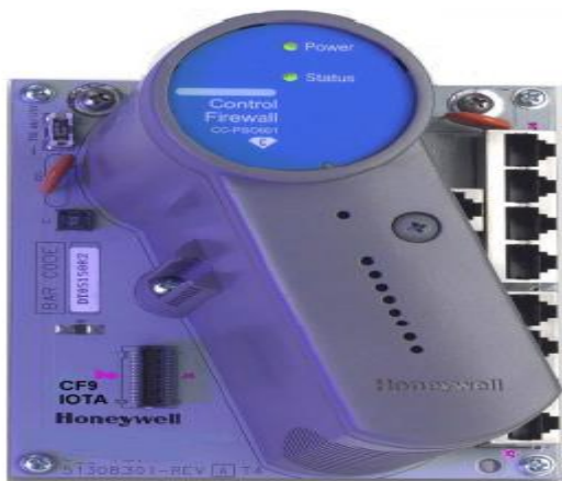
Figure 3.9 : Control firewall CF9
