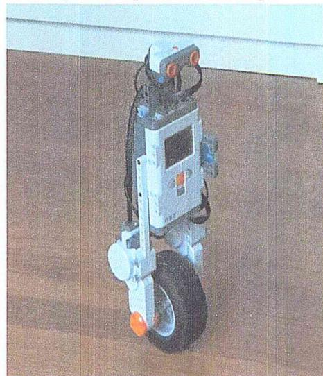
Figure I- 6: Robot Unicycle.
