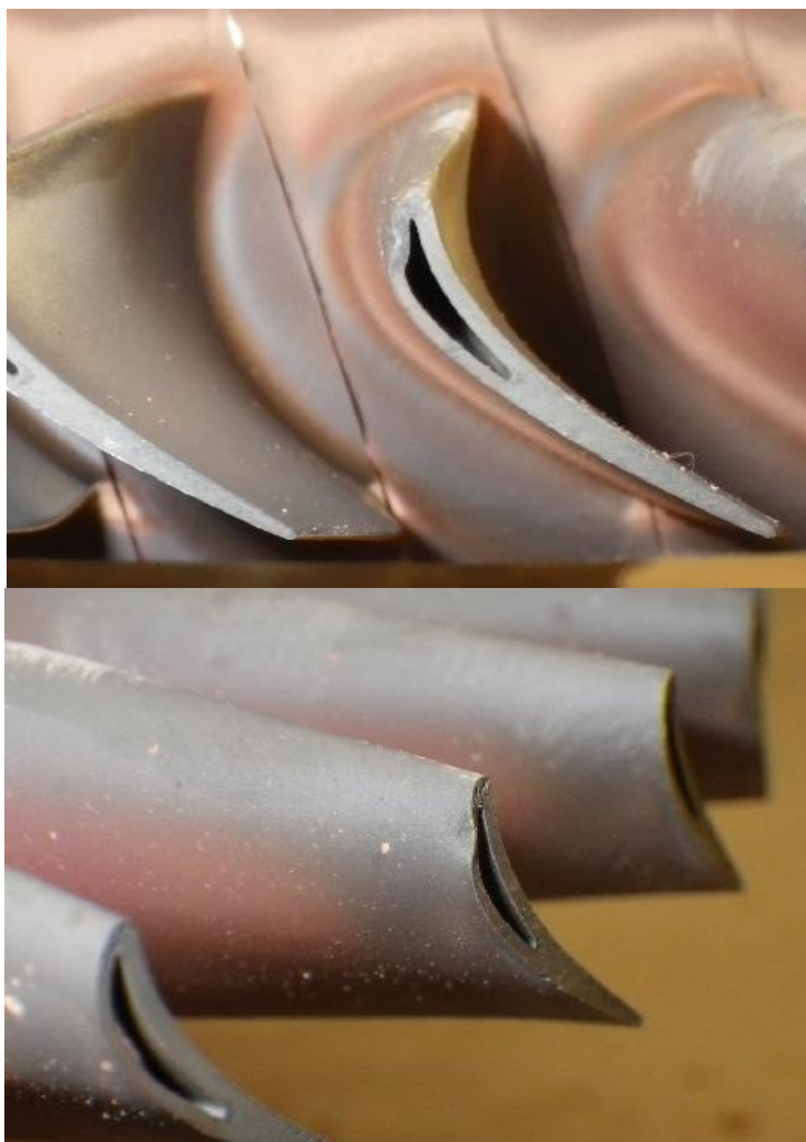
Figure 3.13 - Low pressure turbine blades -
