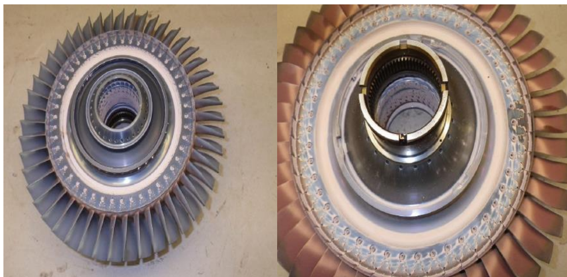
Figure 3.12 - Low pressure turbine blades -
