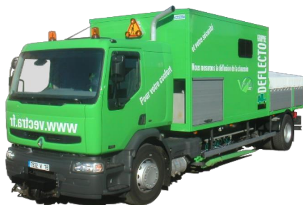
Figure I. 4: Deflectographe Lacroix de NEXTROAD.
