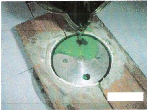
Figure (III.22.a): Coulée de la cire.
