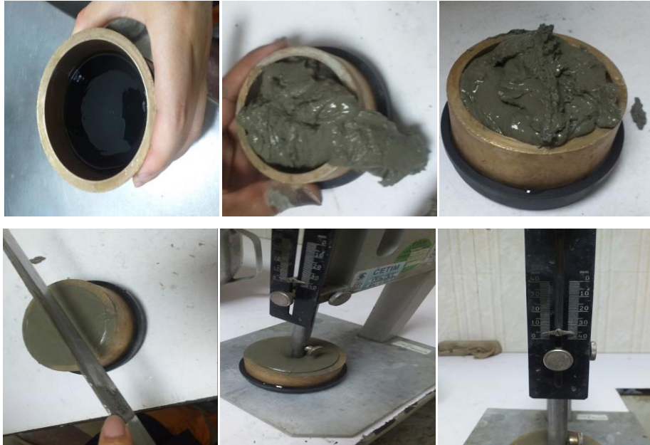
Figure 2.51 : Essai de la consistance normale
