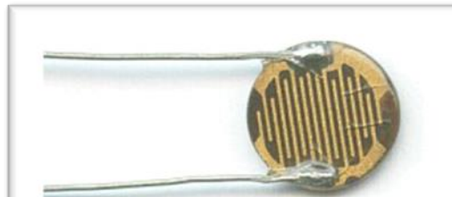
Figure (II- 0:10): Photorésistance LDR
