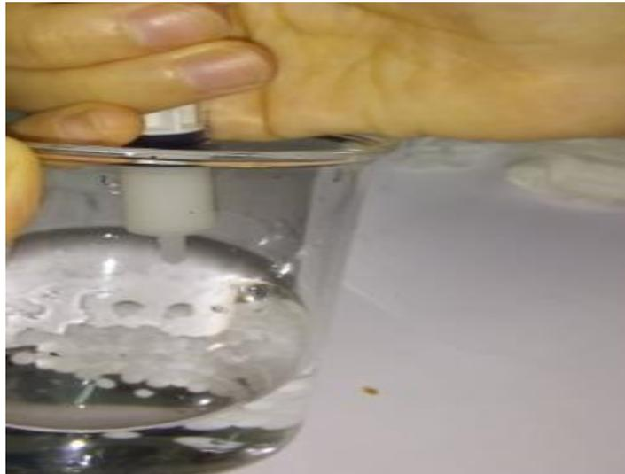
Figure 2.10 Preparation des billes alginate /HDL.
