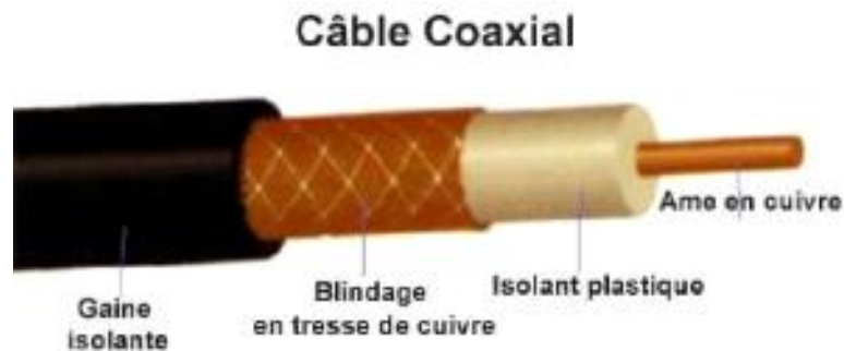
Figure 1. 6 : composition du câble coaxiale.
