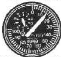
Turbine tachometer (N1 speed)
