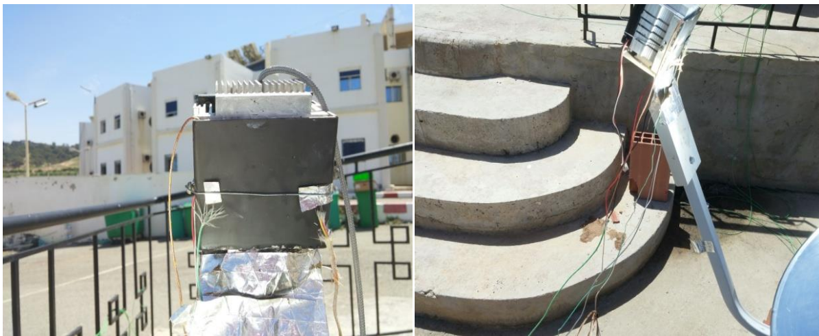
Figure 33: Thermocouples on the measuring points
