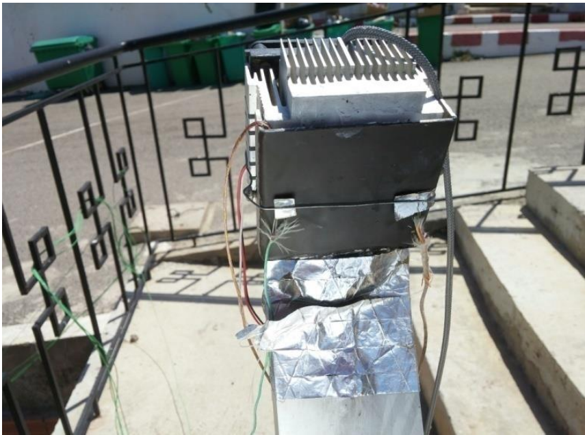
Figure 32: The assembled heat transfer system
