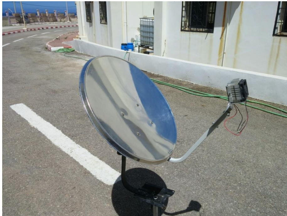
Figure 26: The solar parabolic thermoelectric generator
