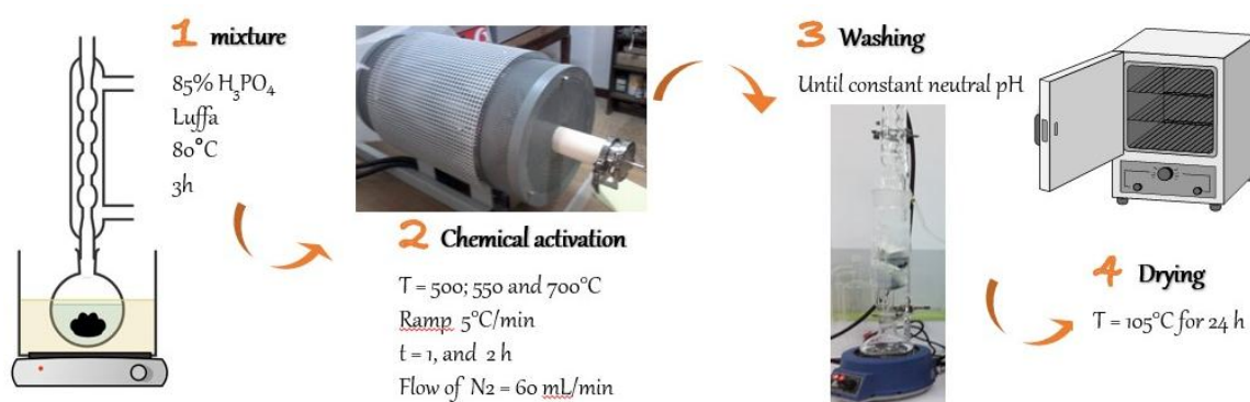
Figure 2.2. Process of Luffa activated carbons preparation
