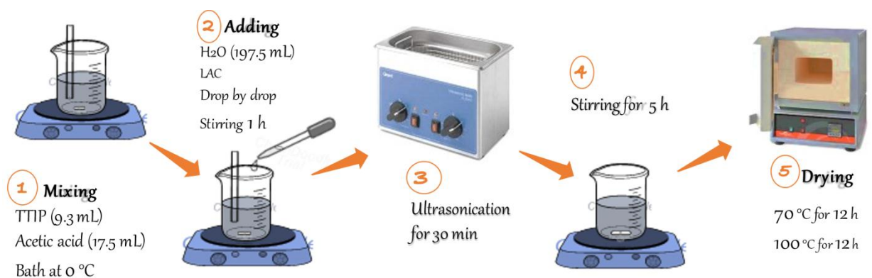
Figure 2.3. TiLAC preparation with Sol-Gel process in presence of acetic acid.
