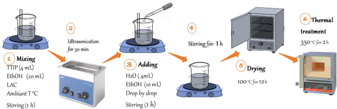
Figure 2.4. Acid-free Sol-Gel process for TiLAC preparation
