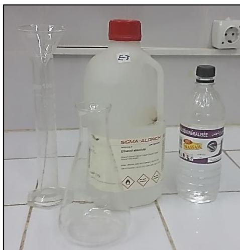
FIGURE 16 MATERIELS DE DILUTION DE L'ALCOOL
