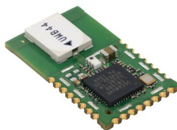
Figure III.10 Le module DWM1000
