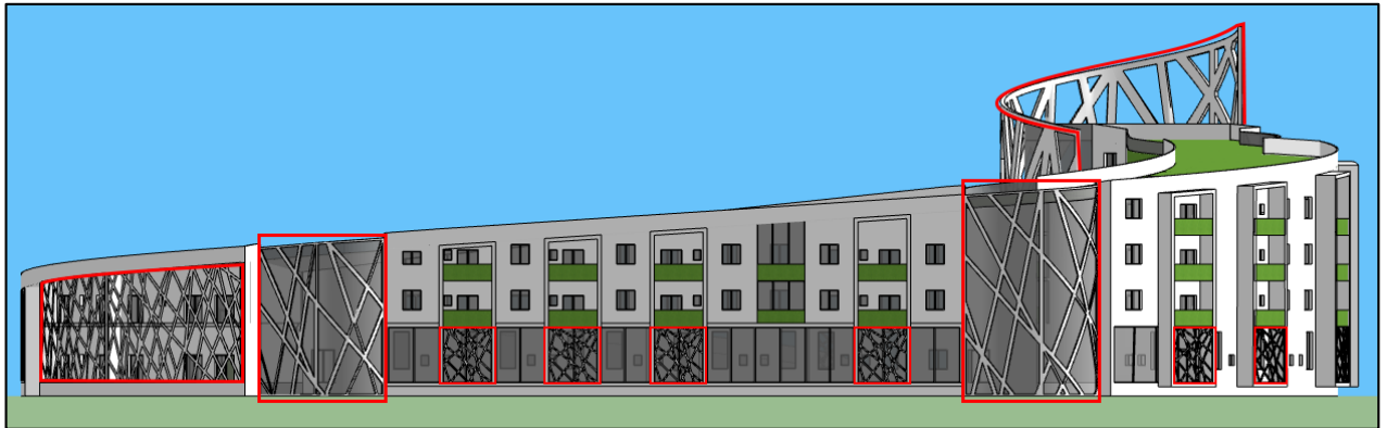
Figure 111 light and sun ray management scheme on the East and the west façade, 1st and 2nd bloc/ source: author
