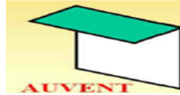
Figure 32: protection solaire type auvent. Source : BELKACEM Nefissa 2017
