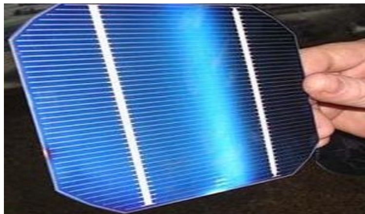
Figure 1. 14. Type de cellule monocristalline.
