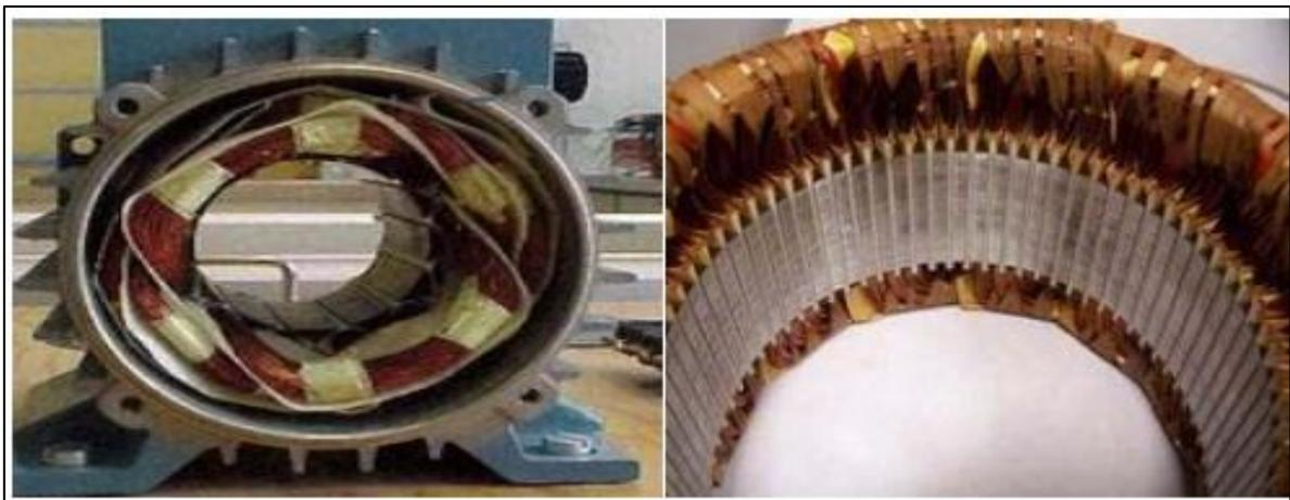
Figure I.4. Le stator.
