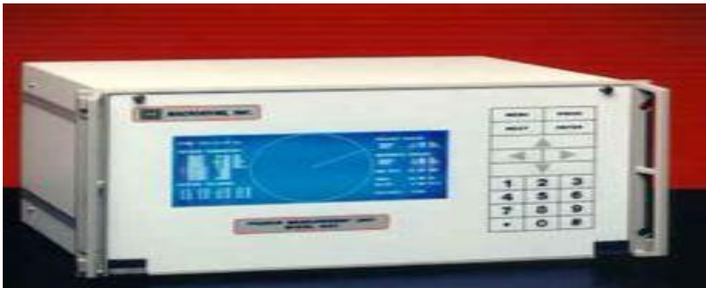
Figure 2.3 : Phasor Measurement Unit (PMU)
