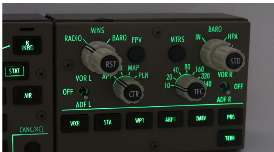
Figure III-2 : EFIS Control Panel
