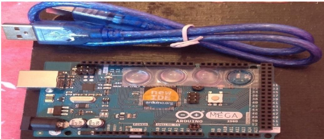
Figure III.18: Arduino + câble USB
