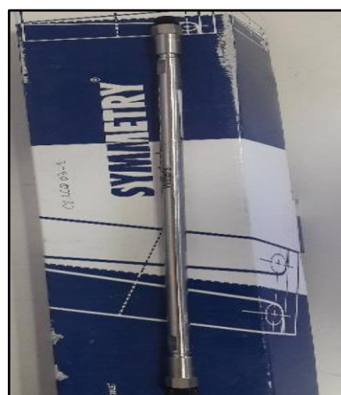
Figure A4 16 : Colonne HPLC type C8 4.6-mm × 15-cm; 5- \mu m emballage L7.
