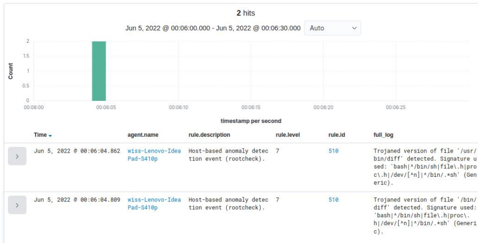
Figure 92: Graphic of the alerts generated by Wazuh in response to the suspicious binary
