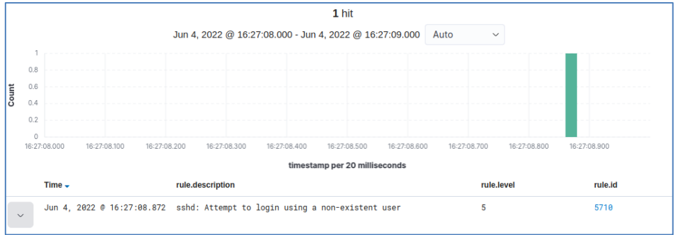
Figure 83: Graphic of the alerts generated by Wazuh in response to the ssh attempt
