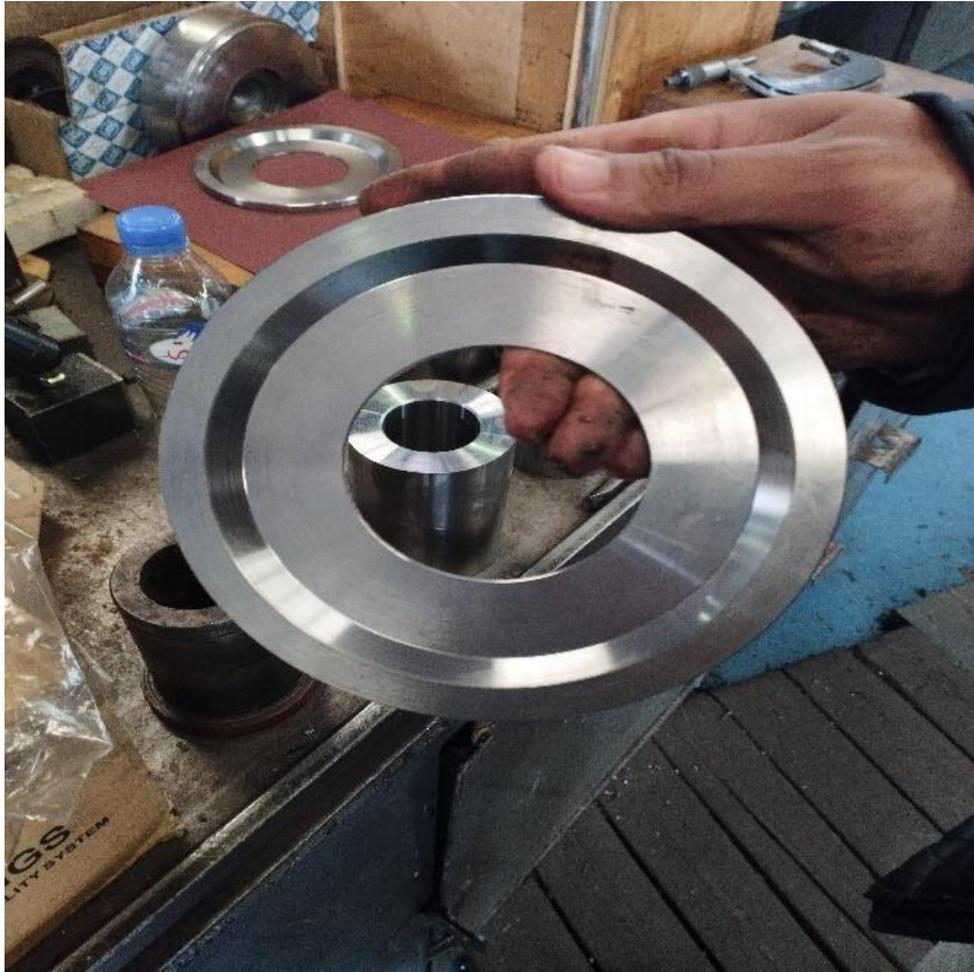
**Figure 5. 22: cache roulement**
