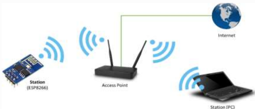
Figure 3.31 : ESP8266 en mode station [12].
