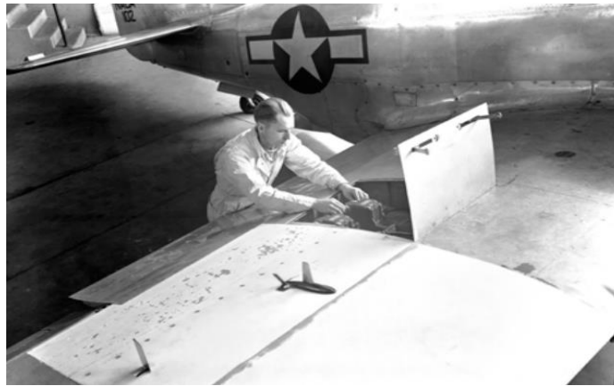
FIGURE I.27. A technician readies the recording instrumentation of a P-51D Mustang modified for wing-flow transonic research. The test model (an XS-1 shape with a swept horizontal tail) is at midspan, with mechanical linkages connecting it to the instrumentation installed within the modified gun bay. NASA Image L-46802 [46]
