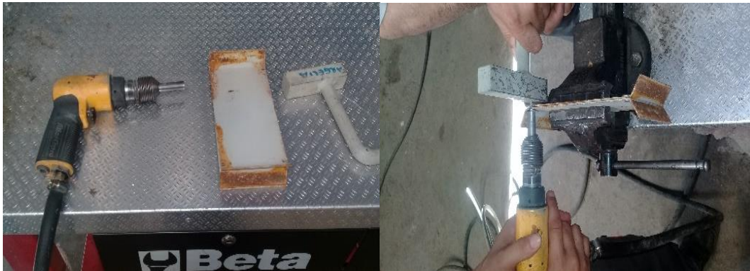
Figure III.3 Making a joint by rivet manually
