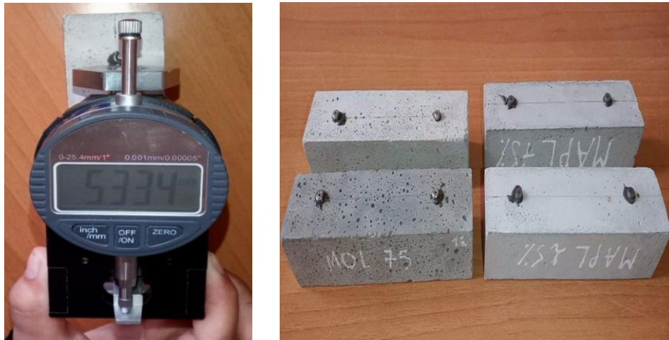
Figure 2.24: Extensometer and specimens with demec gauges
