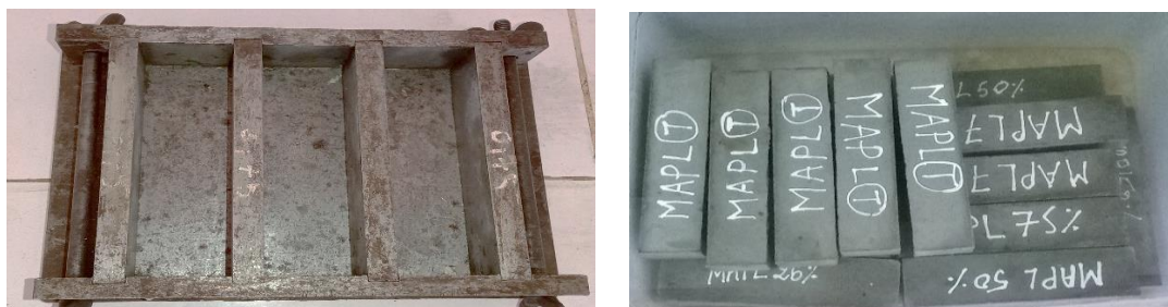
Figure 2.20: Prismatic specimens mould (40x40x160) mm
