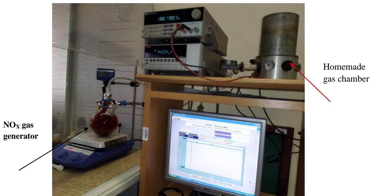
Fig.3.8 Experimental montage for homemade gas chamber
