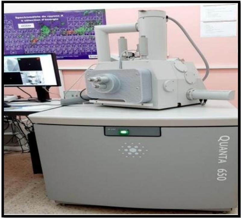
Figure C.5: MEB FEI QUANTA 650.
