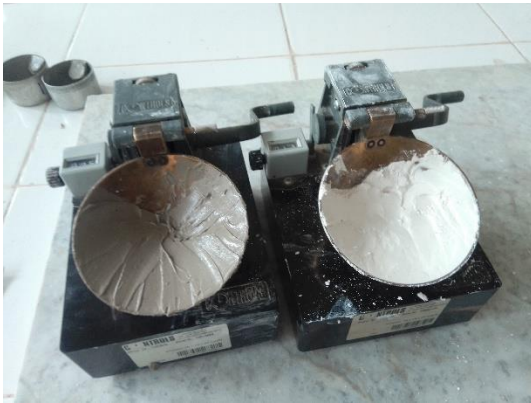
(a) soil pat in the cup of the liquid limit device
