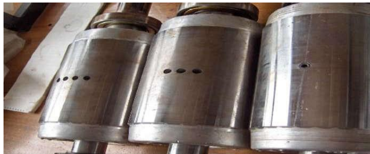
Figure I.8 : Ruptures de barres [9]
