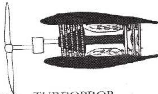
*FIG (1-3)* TURBOPROP
