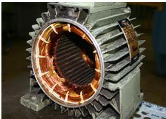
Figure 2.2. Stator [31]
