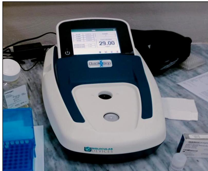
**Figure 37** : spectrophotometer QuikDrop Molecular Devices
