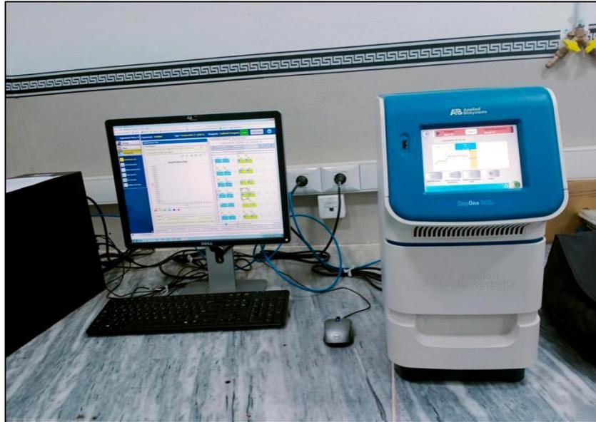
**Figure 36:** Applied Biosystems StepOne Real-Time PCR System
