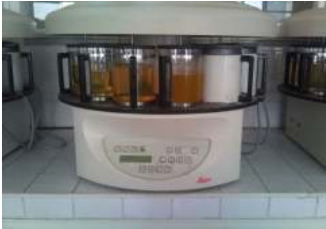
Figure 10: Appareil de circulation
