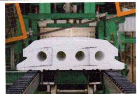
Figure 51 Corps creux polystyrène
