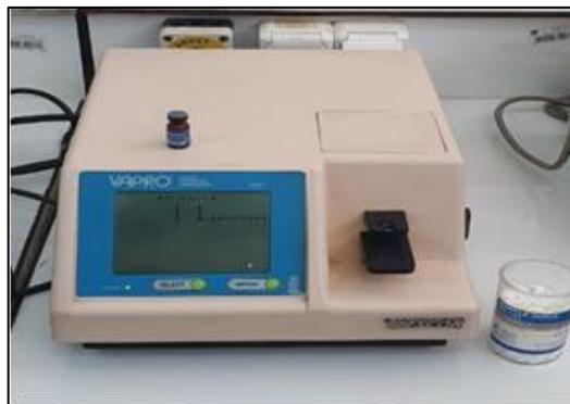
Figure 15: Wescor vapor osmometer VAPRO (model 5520)
