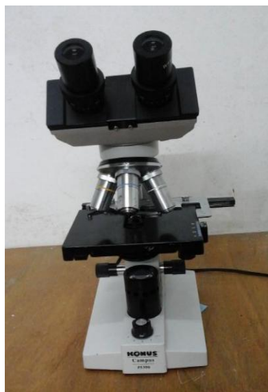
Figure 26: Microscope Konus 5306 Campus (photo originale).
