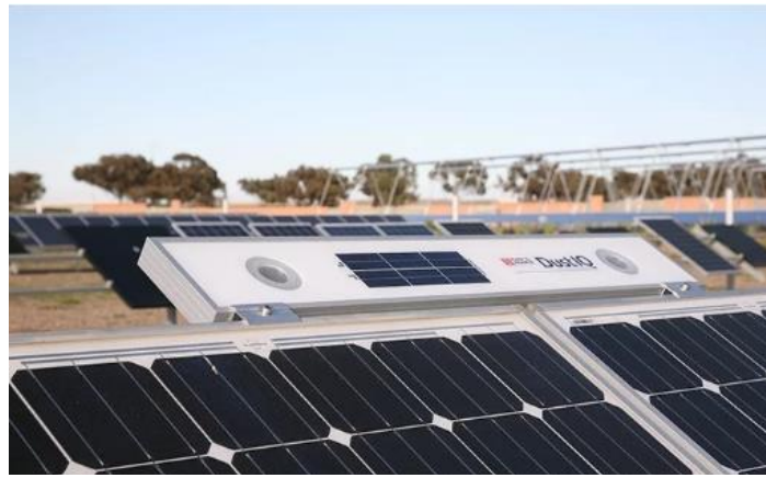
Figure 2.10: DUSST soiling sensor fixed on PV panel [54].
