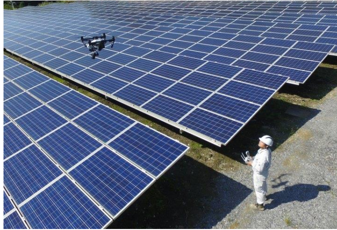
Figure 2.2: Visual inspection using a drone with RGB camera [40].
