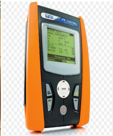
Figure 2.4 : HT Multifunction PV tester [43].
