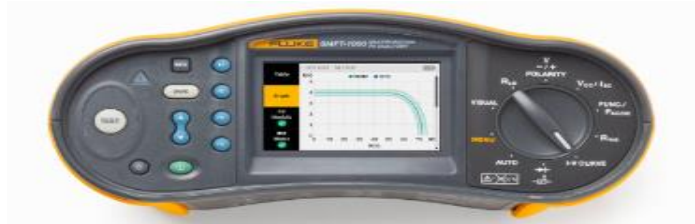
Figure 2.8: I-V Curve tracer & PV multifunction tester
