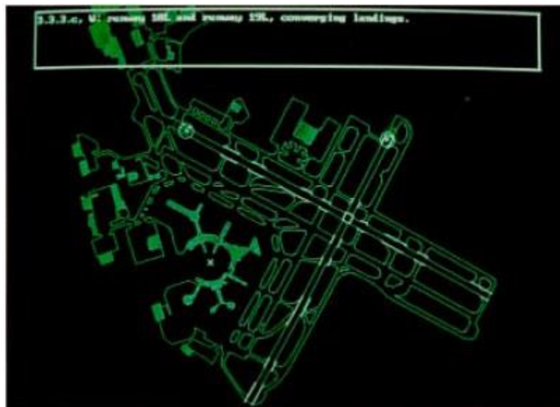
Figure 3-11. Aerodrome movement area safety system (AMASS) display
