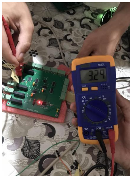
FIGURE 4.3: RTD card power test
