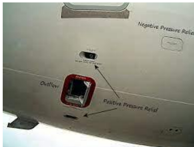
Figure II.4 : soupape de SURPRESSION NÉGATIVE
