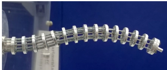
Figure. 1.13: Three-segment continuum robot prototype developed by Bo Ouyang [45].
