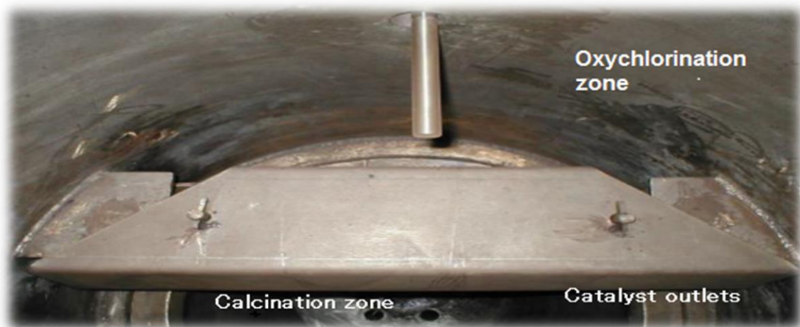
Figure III-4: Zone de calcination
