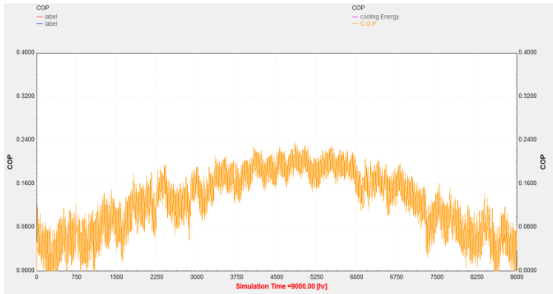
Figure 3-22: variation de COP d'une machine a absorption (Performance Map Collector)
