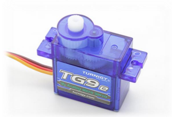
Figure (IV-42). servocommande.
