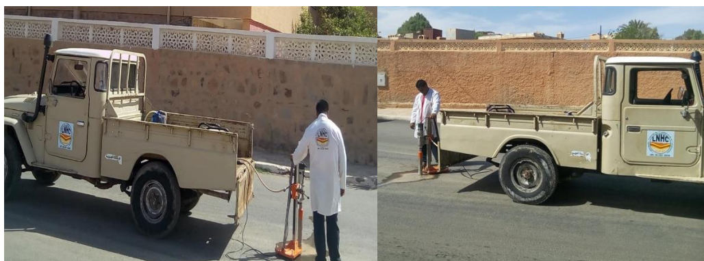
Figure1.15: Photos montrant la dynaplaque2 [7].
